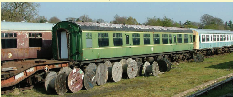
Just a single centre car survives from the Class 120's, unfortunately contaminated with asbestos
