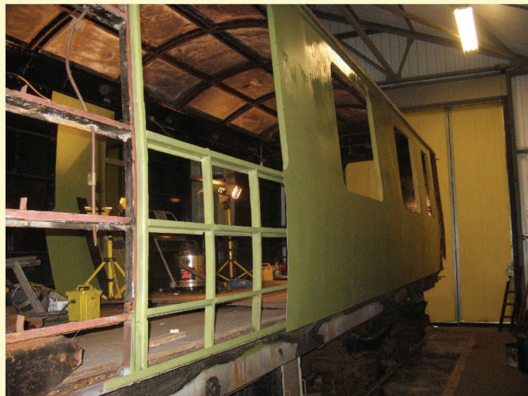
Sc79443 undergoing major bodywork repairs, 11/3/12 (J.Horne)
